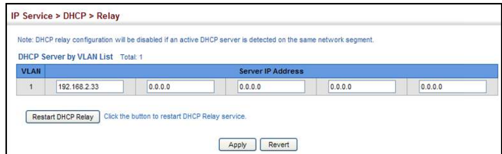
Figure 423: Configuring DHCP Relay Service
