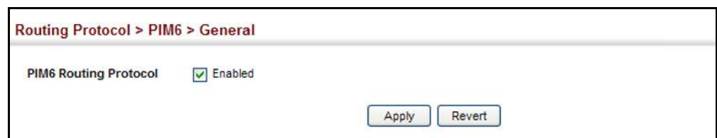
Figure 534: Enabling PIMv6 Multicast Routing
