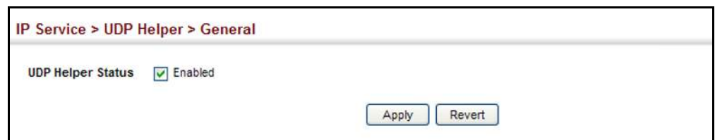
Figure 432: Enabling the UDP Helper
