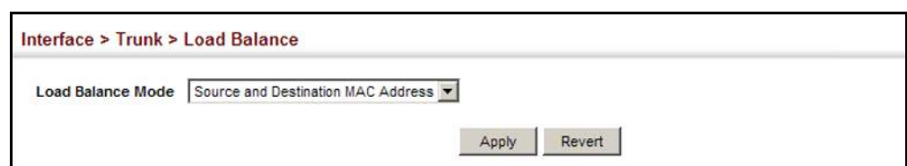
Figure 62: Configuring Load Balancing
