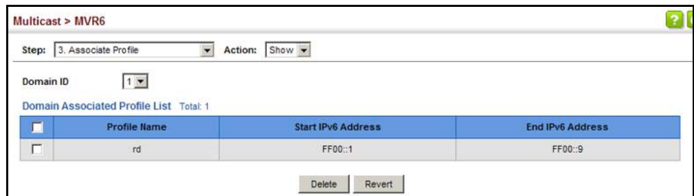
Figure 391: Showing MVR6 Group Address Profiles Assigned to a Domain
