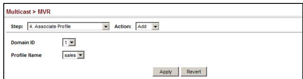
Figure 377: Assigning an MVR Group Address Profile to a Domain
