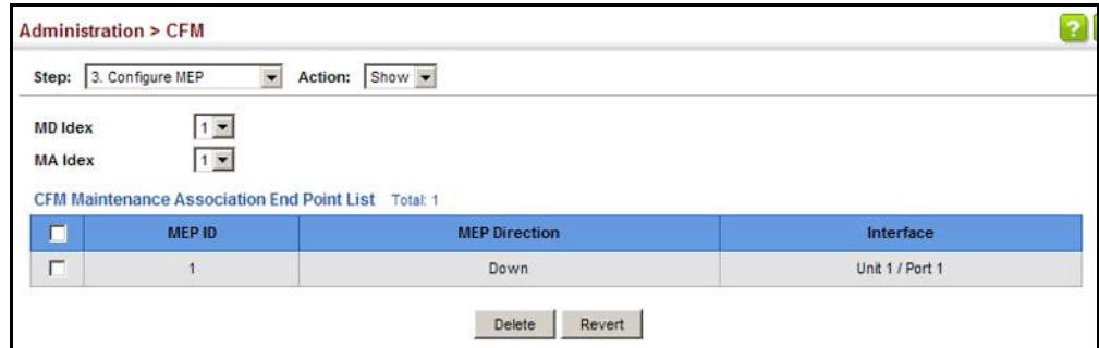
Figure 313: Showing Maintenance End Points
