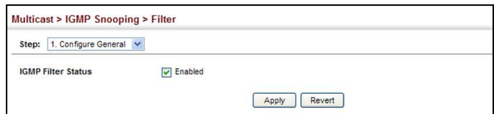
Figure 350: Enabling IGMP Filtering and Throttling
