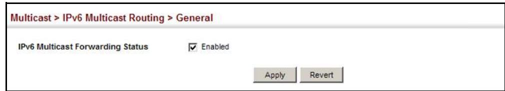
Figure 517: Enabling IPv6 Multicast Routing
