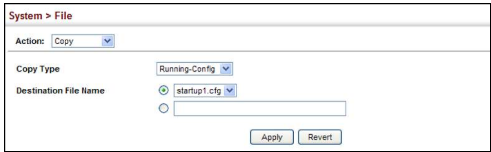
Figure 8: Saving the Running Configuration
