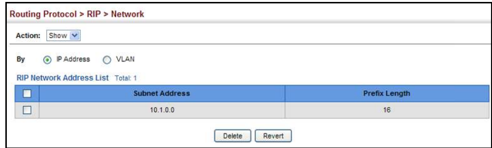
Figure 468: Showing Network Interfaces Using RIP
