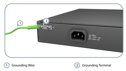
Before powering on the switch, ground the switch to earth as described below.
