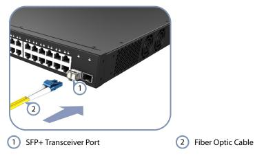
**4.** As a connection is made, check the Link LED on the switch to be sure that the connection is valid.
