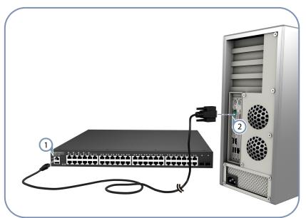
(1) Connect console cable to switch's Console port.
