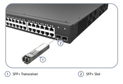
**Note:** To remove a transceiver: First disconnect the network cable, then pull the tab to remove the transceiver from the slot.
