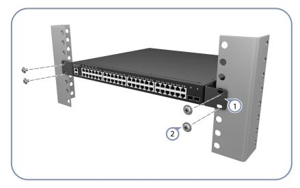
1 Attach the brackets to the switch.
