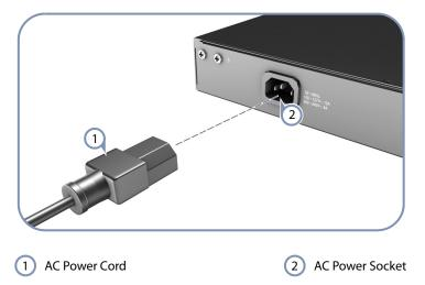
**2.** Insert the plug on the other end of the power cord directly into the AC input socket on the back of the switch.
