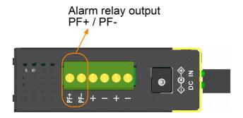
Use the provided 2P terminal plug for signal wiring and plug into the PF+/- contacts.
