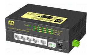
For more coming PoE (Power Over Ethernet) applications, the PoE switch model is equipped with PoE design in four copper ports. With proper 48VDC power supply, it is able to deliver power to four PoE PD devices via Cat.5 cables. This guide describes the installation information about two models as follows:
