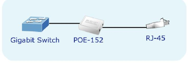
Figure 1: the Injector installation
