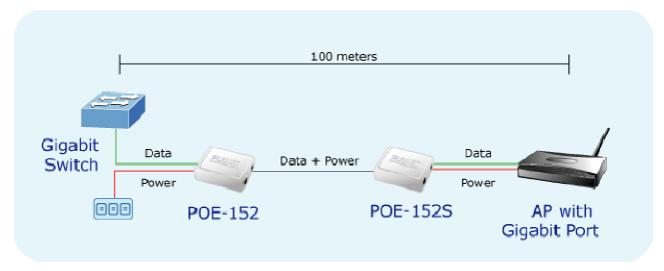
Figure 3: Connection architecture over POE-152/152S
