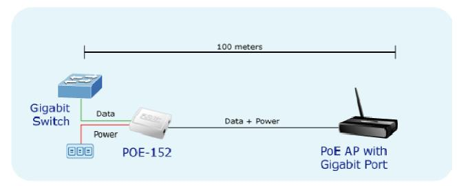
Figure 4: Connection to IEEE 802.3af device
