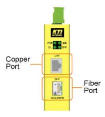
Copper port is featured to support connection to:
