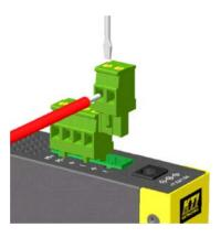
If cascading the power to next device is needed, install the power wires and plug for another switch. Then, use DC2 contacts.
